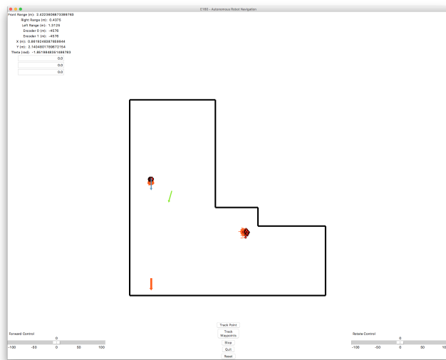
Fig. 9: The E160 graphical user interface. The GUI displays the map (walls colored black), the estimated odometry state (orange arrow), the estimated particle filter state (light-green arrow), the desired state (orange arrow), and the particles (red circles).
